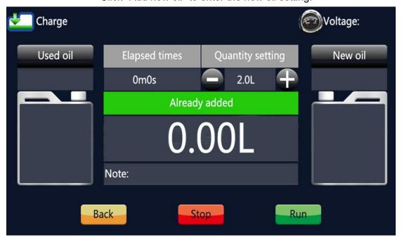
Set the required amount of replenishment on this interface before adding new oil, and press "Run".
